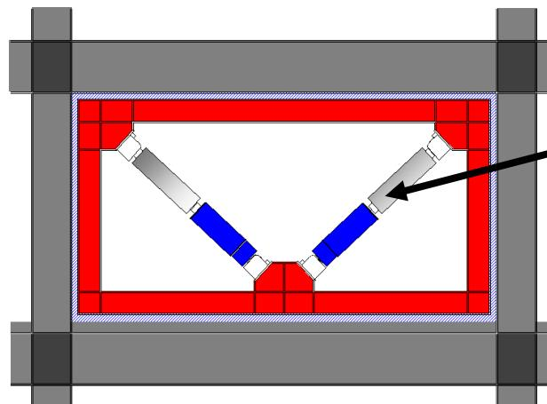
**Oil damper with the controlled axial force**
