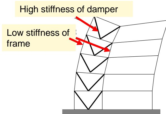
Flexural deformation of main frame
