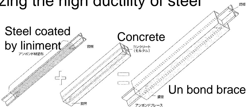
Buckling restrain brace
