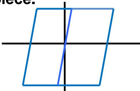
Normal bilinear force characteristics of friction damper
