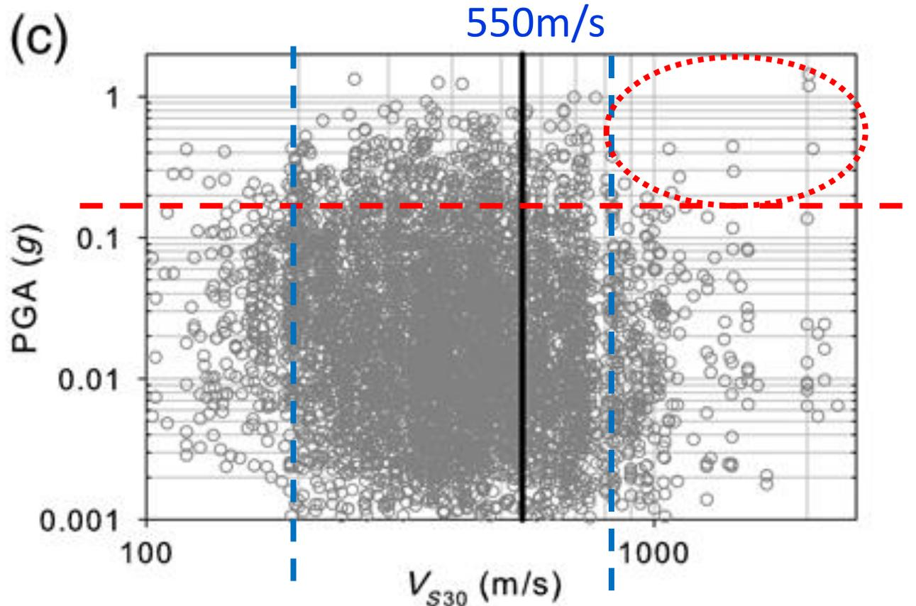
Poor and loose data distribution for hard-rock conditions and  $PGA > 0.20g$
